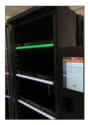
Now fill in the weight of the calibration tool that got delivered together with the fridge (1000g). Press NEXT.
